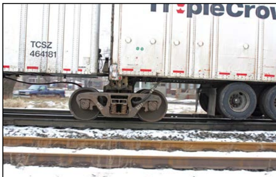
Figure 2.47; Piggyback trailer system.
