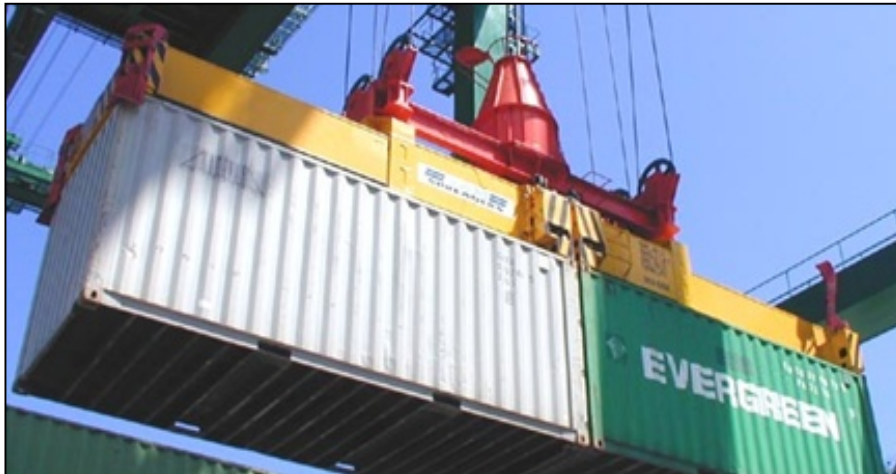
Figure 2.55; Container spreader; lifting device that hooks into the corner castings of a container.
