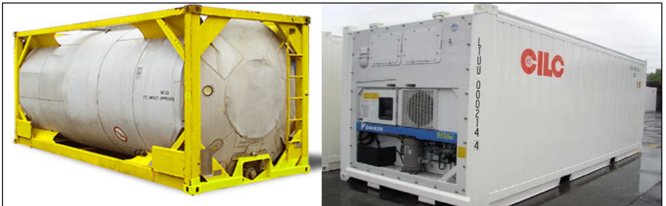
Figure 2.42; Left; Tanktainer for liquid bulk. Right; Reefer for refrigerated cargo.
