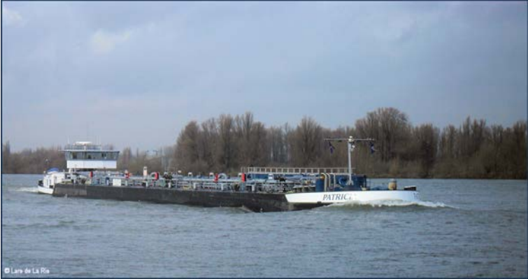
Figure 2.49; River transport of liquid bulk by a tanker barge.
