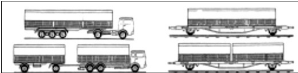
Figure 2.41; Swap-bodies on road and rail transport.
