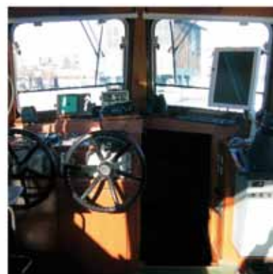
Mandatory vessel equipment with an optional ECDIS viewer in Austria
