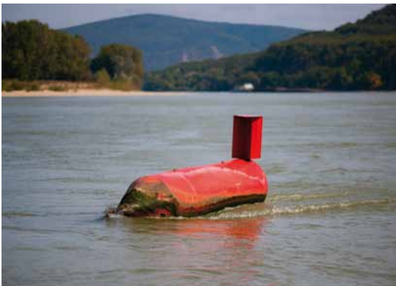
Red buoy with cylindrical topmark for marking the right-hand fairway limit
