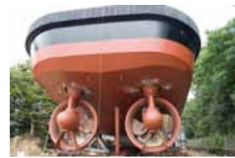
Twin-screw propulsion with ducted propellers
