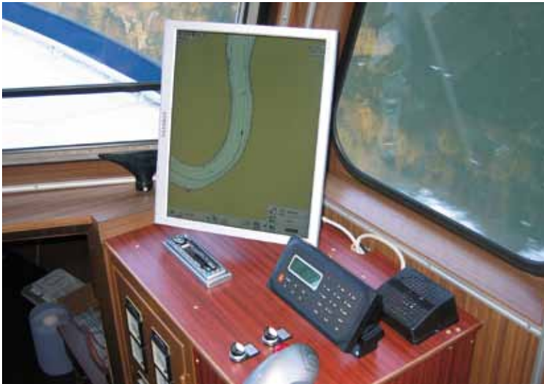
Electronic navigational chart in support of navigation
