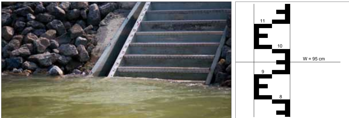
Gauge staff at a gauging site; sample water level at gauge: 95 cm
