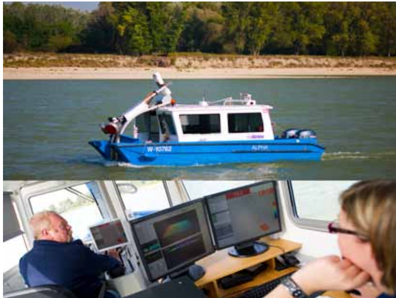
Multi-beam riverbed survey on the free-flowing section of the Danube east of Vienna by via donau – Österreichische Wasserstraßen-Gesellschaft mbH
