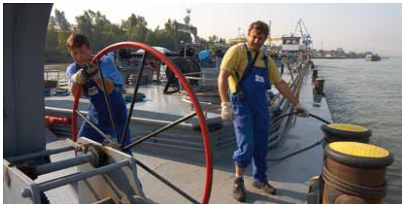
Crewmen connecting a tank lighter
